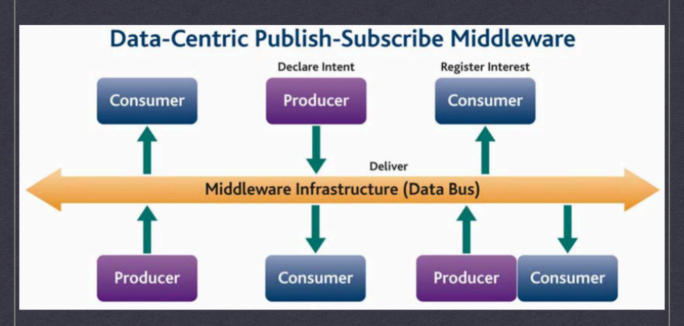
A DDS application is composed of data providers & consumers, each potentially on different computers.
