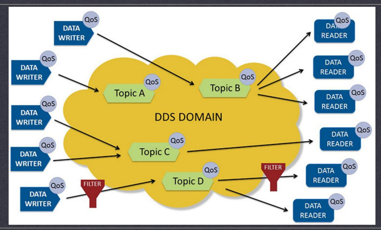
DDS provides QoS-controlled data-sharing. Subscriptions can specify time and content filters and get only a subset of the data being published on the Topic.
